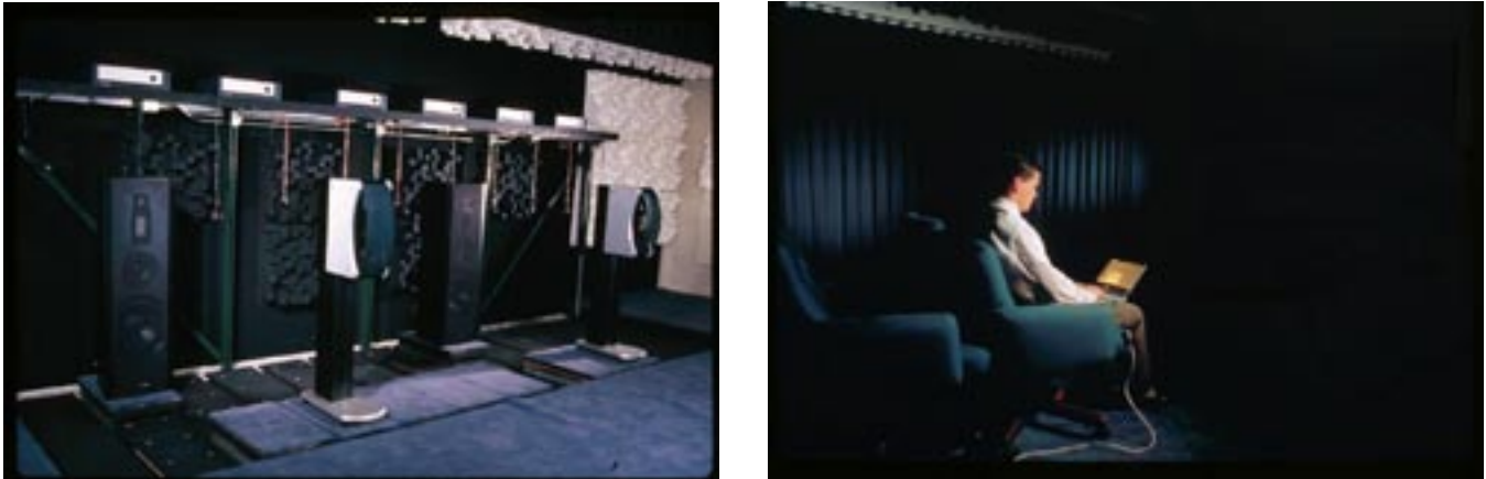
Figure 13. A computer-controlled, pneumatically-operated loudspeaker mover eliminates loudspeaker position as a variable in listening tests. The photo on the left shows one stereo pair of loudspeakers in the active location, while another pair is parked quietly against the back wall. The listener controls the test, switching among the comparison loudspeakers while forming opinions (there can be up to four single loudspeakers, four stereo pairs, or three L,C,R combinations). Of course the tests are double-blind.
