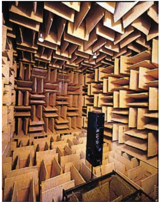
Figure 15. A 4\pi (full space) anechoic chamber in which high-resolution measurements over the entire audible bandwidth are possible. This chamber is naturally anechoic down to 60 Hz, and calibrated down to 20 Hz. The platform on which the loudspeaker is located rotates to permit measurements over a full 360^\circ orbit. The loudspeaker is then tilted to complete orbits over more of the total sphere surrounding it.
